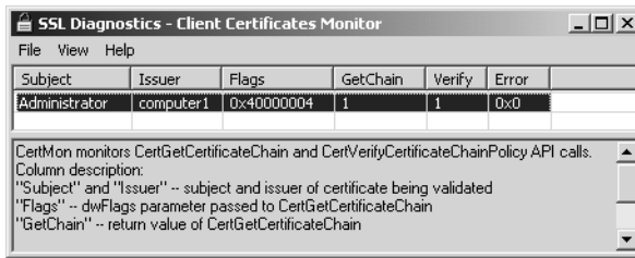
Figure 11.7 The SSL Diagnostic Utility monitoring client certificates
